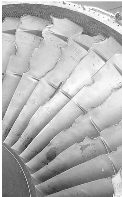
The result of FOD—a damaged engine.
