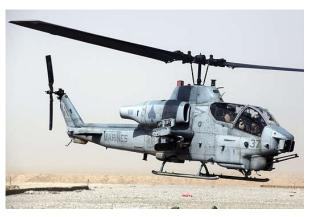
According to a U.S. Marine accident report, the fatal crash of a Marine AH-1 attack helicopter in California last year was caused by a collision with a female red tailed hawk. This raptor, weighing about 3 pounds (1.5 kg), apparently struck the AH-1 just below its rotor blades on part of the transmission know as the pitch change link. The rotors became unbalanced and the aircraft broke into 3 sections almost immediately. Both Marine aviators were killed on impact.
