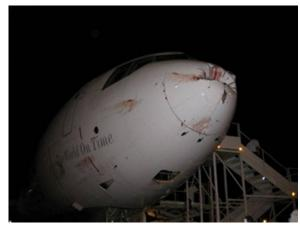
Largely unnoticed and certainly uncommented upon was the near disaster suffered by a Fedex MD-11 upon departure from Memphis, Tennessee on March 1st. During the late night departure, while climbing through about 8,500°, the aircraft struck a flock of snow geese. The aircraft was extensively damaged according to the Fedex report. The report noted that all three engines were struck by geese; two of the three engines ingested geese and were damaged or essentially destroyed. Further, the geese pene-
